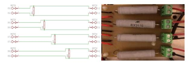
Resistor Board PCB schematic
